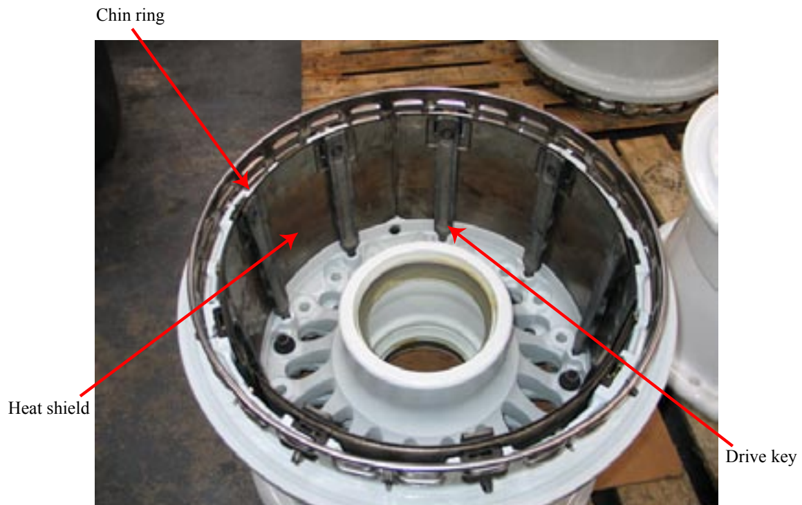
Figure 4 Construction of main wheel
