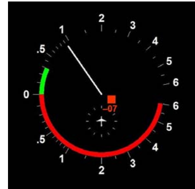
Figure 9: A weakening “Level off, level off” RA as shown on a generic IVSI display
