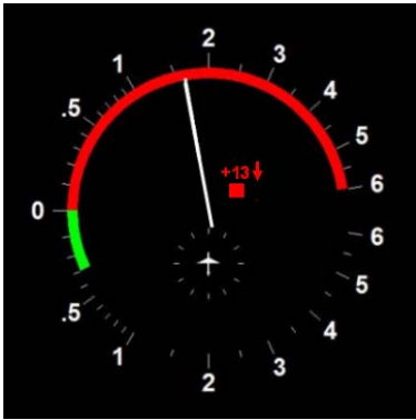
Figure 7: “Level off, level off” RA as shown on a generic IVSI display
