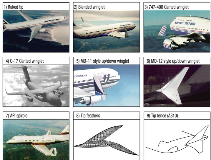
*Figure 1.1. An assortment of wingtip device configurations*
