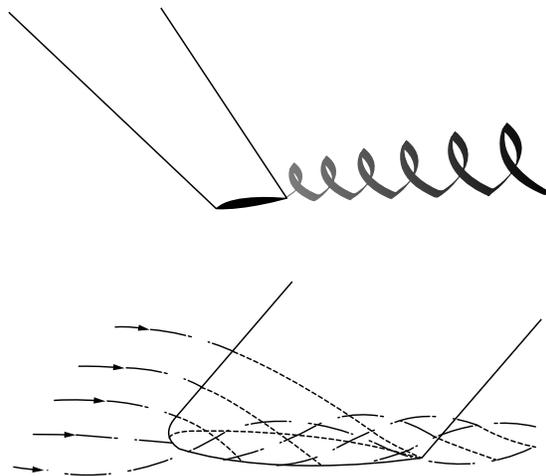
Figure 3.3. Misleading views of a compact "wingtip vortex"
