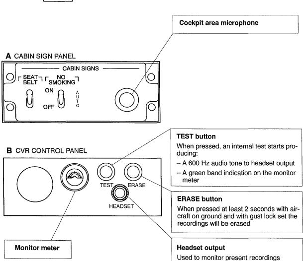
FIG.1. Cockpit voice recorder - controls and indicators.
