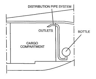
FIG.6. Cargo fire controls.
