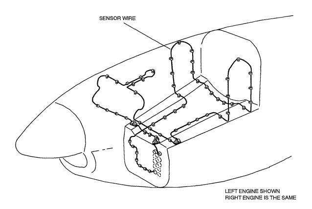
FIG.2. Engine fire detection sensor.
