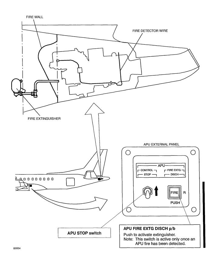
FIG.5. APU external controls, fire detection and extinguishing.
