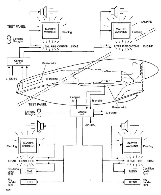
FIG.1. Engine and tailpipe detection schematic.
