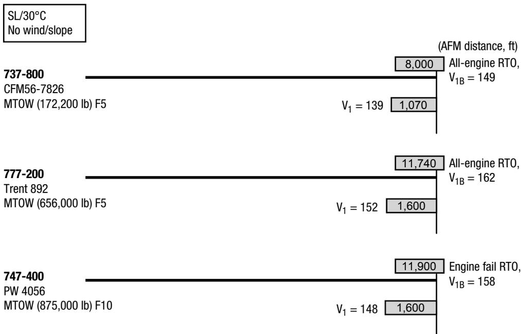
Figure 6. Accelerate-stop margins; RT0 10 knots prior to V<sub>1B</sub>, dry runway
