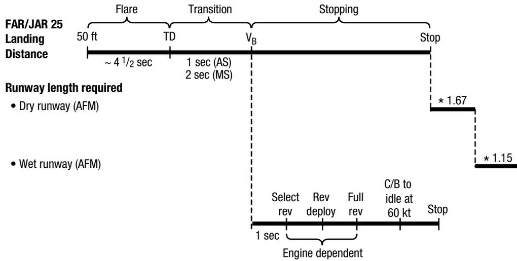
Figure 11. Landing distance calculation basis
