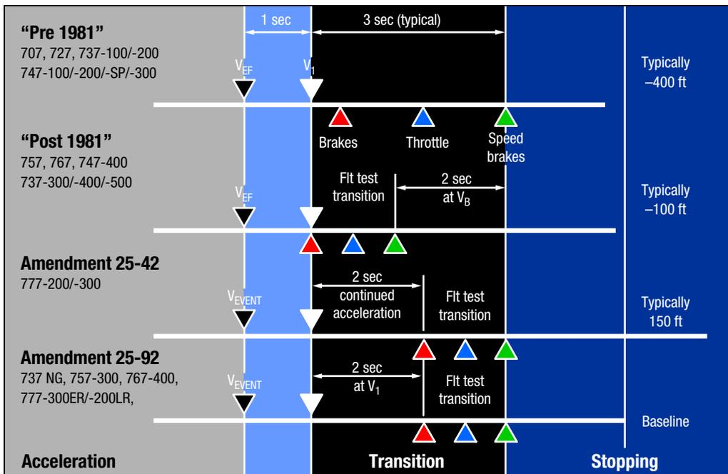
Figure 2. Accelerate-stop transition segments
