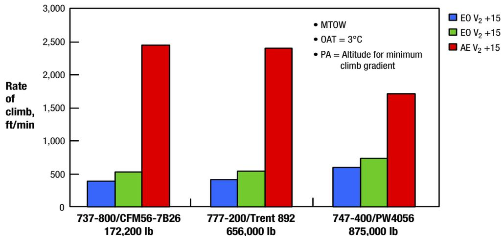
Figure 8. Rate of climb capability second segment limit
