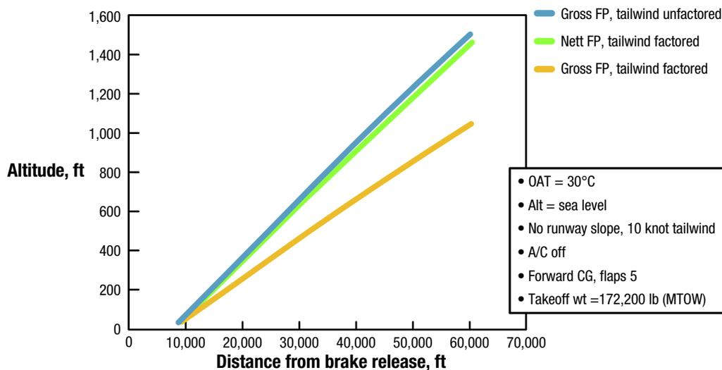
Figure 10. 737-800/CFM56-7B26 takeoff flight path
