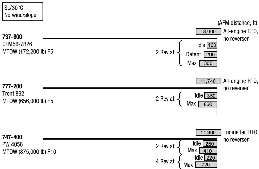
Figure 4. Accelerate-stop margins; thrust reversers, dry runway
