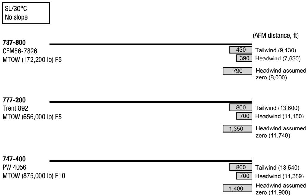
Figure 3. Accelerate-stop margins; wind accountability (10 knots), dry runway
