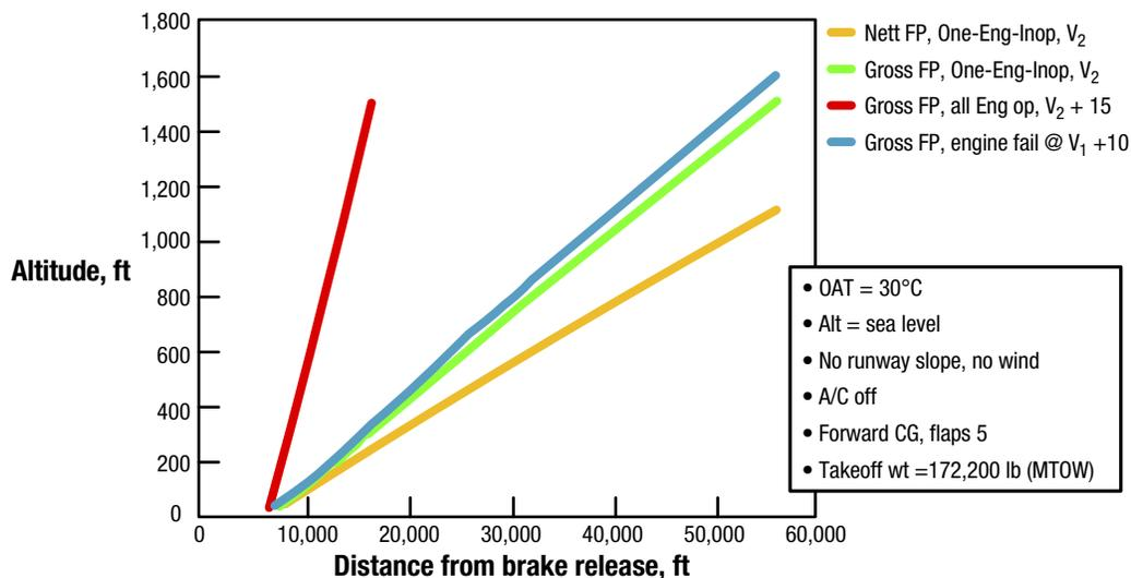
Figure 9. 737-800/CFM56-7B26 takeoff flight path
