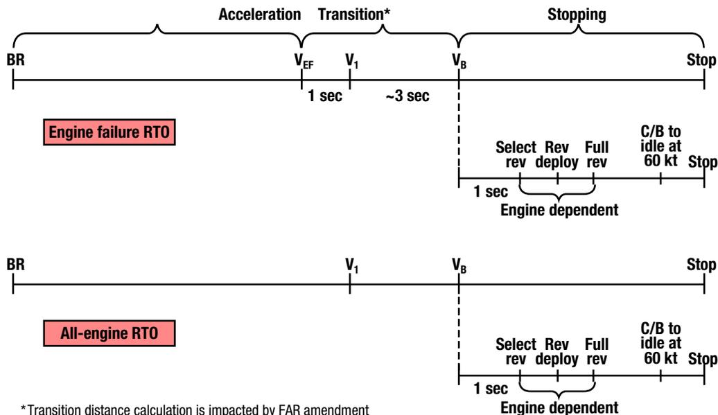
Figure 1. Accelerate-stop distance calculation basis
