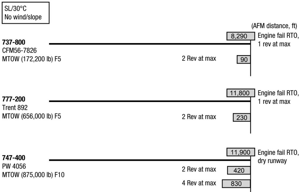
Figure 5. Accelerate-stop margins; thrust reversers, wet runway
