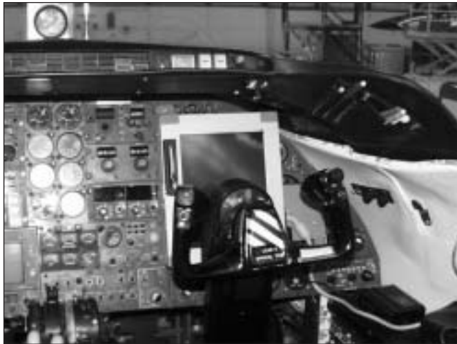
The right seat instrument panel of the Learjet 25B variable-stability in-flight simulator has an electronic visual display with attitude director indicator (ADI) and airspeed and altitude vertical readouts. Other controls, such as flaps, and other displays, such as engine monitors, are standard Learjet equipment. (Photo:U.S. National Aeronautics and Space Administration)
