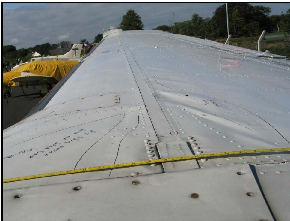
Photo 2 Upper skin rippling on starboard wing outside outer wing panel joint
