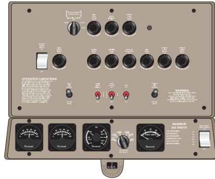
OVERHEAD LIGHT CONTROL PANEL
