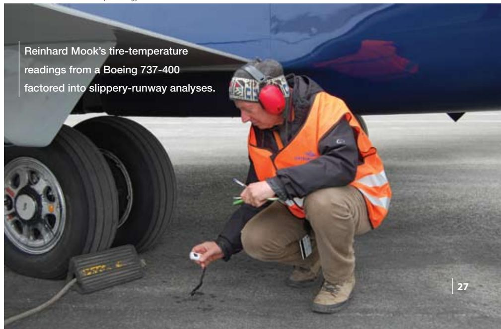
Reinhard Mook's tire-temperature readings from a Boeing 737-400 factored into slippery-runway analyses.
