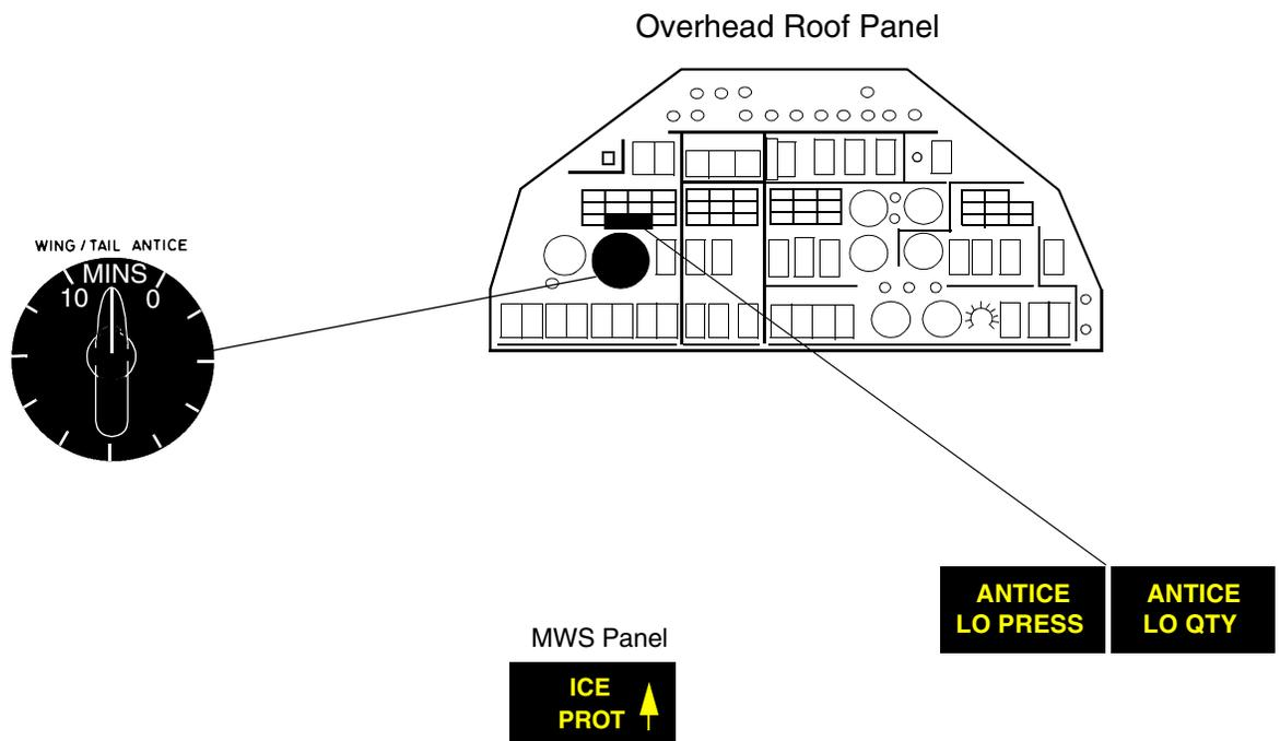
**NOTE:** At very low temperatures (-28° C or less) ice crystals can exist in the atmosphere, but do not present a hazard. If the airframe ice protection system is used at these low temperatures, the water/alcohol content of the fluid will evaporate, leaving solidified glycol which together with the impinging ice crystals can give the appearance of ice. Use of the airframe ice protection system, under these conditions, is not advisable.
