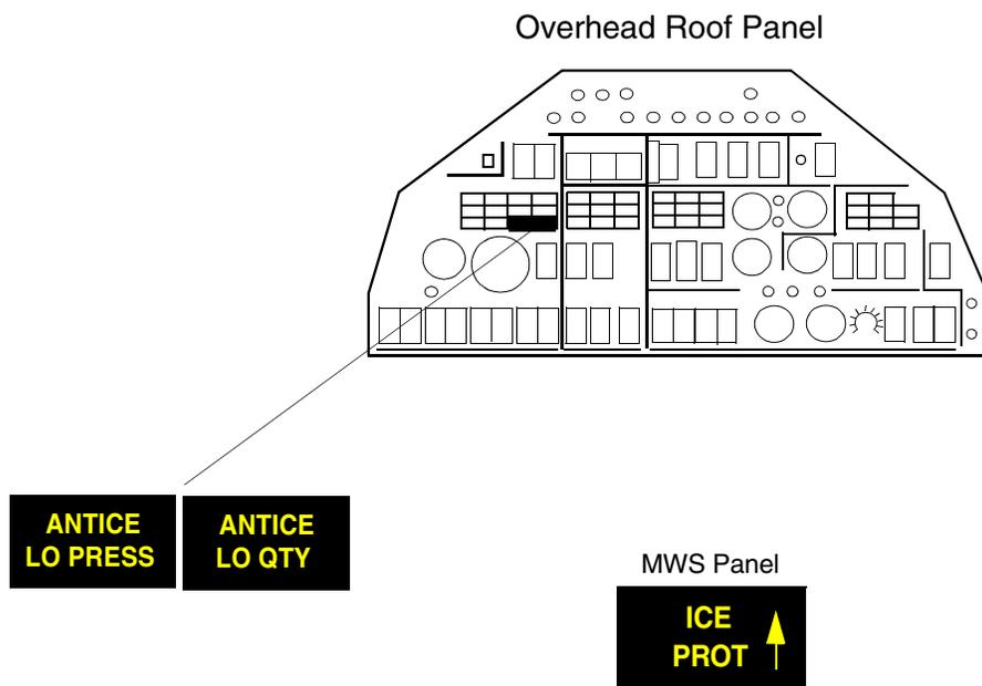
Fluid low quantity is indicated by the illumination of an amber ANTICE LO QTY annunciator on the overhead roof panel and the MWS ICE PROT repeater annunciator flashing. When these warnings occur, 30 minutes of fluid usage remains.
