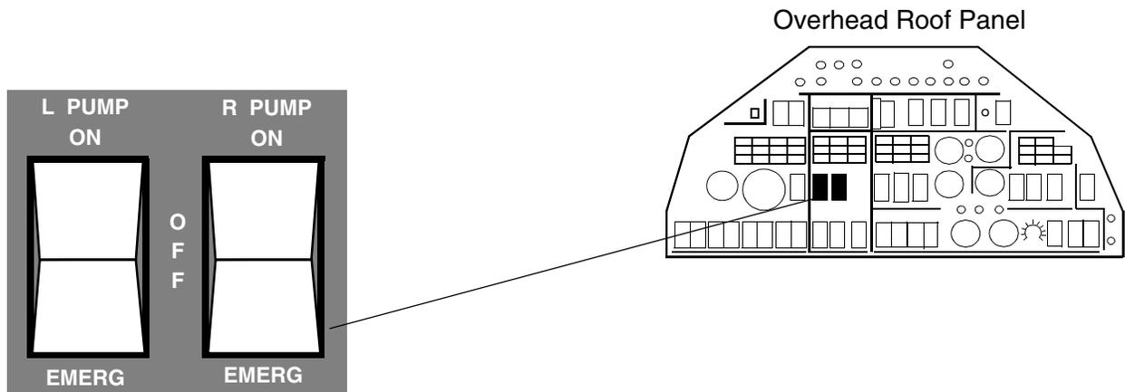
Should both fuel pumps fail, fuel still gravity feeds into the fuel reservoir of each wing so that the engine driven pumps can draw the fuel for operation under suction feed. Warning of pump failure is provided by a FUEL 1 LO PRESS and/or FUEL 2 LO PRESS amber annunciator located on the overhead roof panel. To alert the flight crew of these warnings, these annunciators are accompanied by a flashing repeater annunciator located on the MWS panel.
