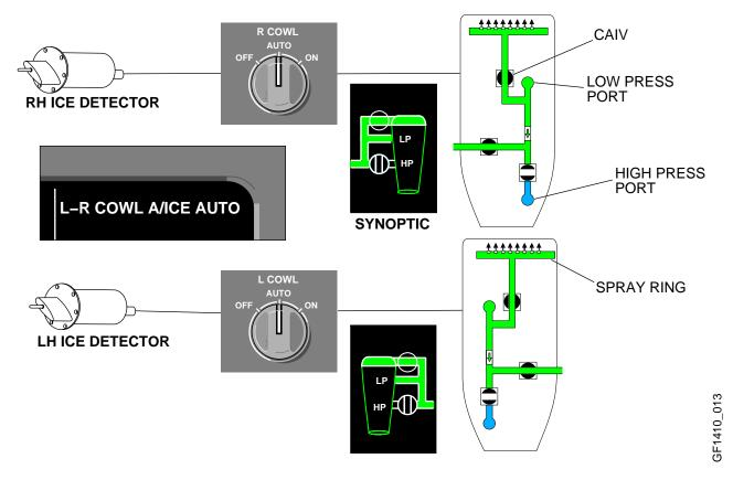
Cowl anti-icing can be manually selected to ON, in which case the CAIVs will open, independent of the ice detection system and a status message is displayed. Whenever cowl anti-ice is activated (AUTO or ON), a CAI icon will be displayed on the EICAS page.
