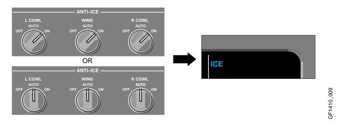
If both ice detectors are failed, a message is displayed on EICAS and the crew must revert to manual selection of cowl and wing anti-ice.
