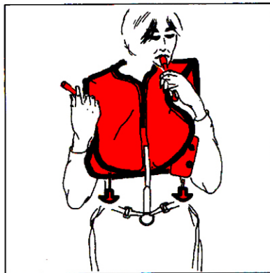
7. Should it become necessary, life vest can be orally inflated by blowing into oral inflation tubes.
