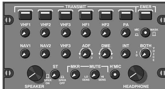
Audio Control Panel
