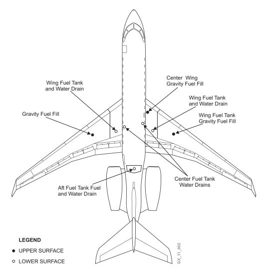
All tanks have flush self-closing water drain valves, installed at various low points, to permit draining of any accumulated water or residual fuel. They are located at the low point of each wing. Three gravity fill caps are provided for wing and center tank gravity refueling.
