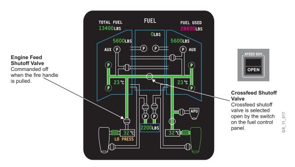
A secondary use of the crossfeed system (as a back-up to the wing transfer system) is to provide means of correcting lateral C of G imbalances, by temporarily inhibiting the flow of fuel from the light side of the airplane. Fuel will then be supplied to both engines from the "heavy" side until lateral fuel balance is within desired limits.
