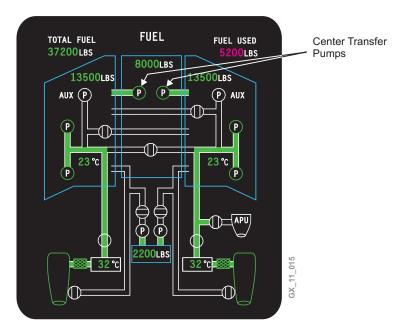
The FUEL synoptic page represents the center tank transfer system in operation, with both engines running.
