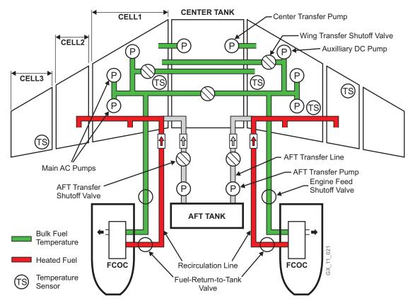
The wing fuel tanks are fitted with many fuel temperature sensors; the left wing has two and the right wing has three. With the Fuel Recirculation OFF, the Fuel Management and Quantity Gauging Computer (FMQGC) reads all temperature sensors but will display only the lowest temperature. When the Fuel Recirculation system is ON, the FMQGC computer reads the inboard temperature sensor as it will be the one who reads the highest temperature.
