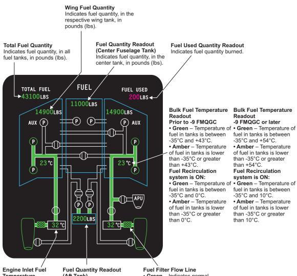
Engine Inlet Fuel Temperature • Green – Engine fuel temperature is  $\geq 5^{\circ}$ C. • Amber – Engine fuel temperature is < 5^{\circ}C. Fuel Quantity Readout (Aft Tank) Indicates fuel quantity in the aft tank, in pounds (lbs). Fuel Filter Flow Line • Green – Indicates normal fuel flow to the engine. • Amber – Fuel pressure drop exists across the filter, flow line from the filter to the engine turns amber.
