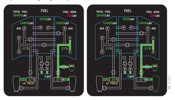
The FUEL synoptic page below represents airplane configuration with the APU shut down, both engines on, the AC pumps running, and the DC pumps on standby.
