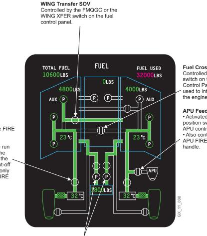
AFT Tank Transfer Valve Controlled by the FMQGC or the AFT XFER switch on the fuel control panel.
