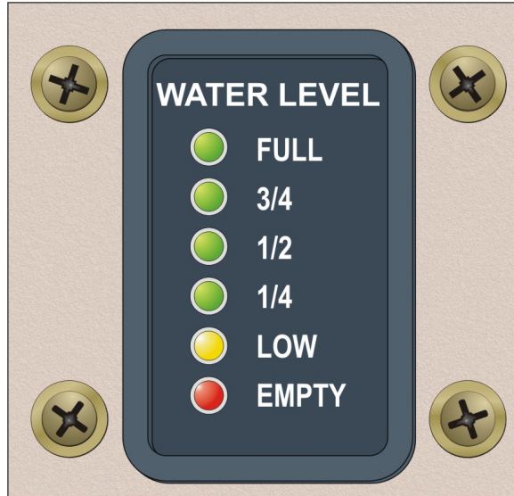
FIGURE 02-38-20-04 - WATER LEVEL INDICATION
