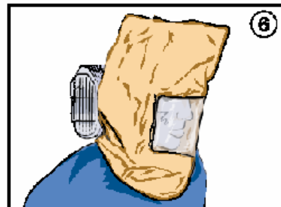
THE SOLID STATE OXYGEN GENERATOR ENSURES A MINIMUM FLOW FOR 15 MN
