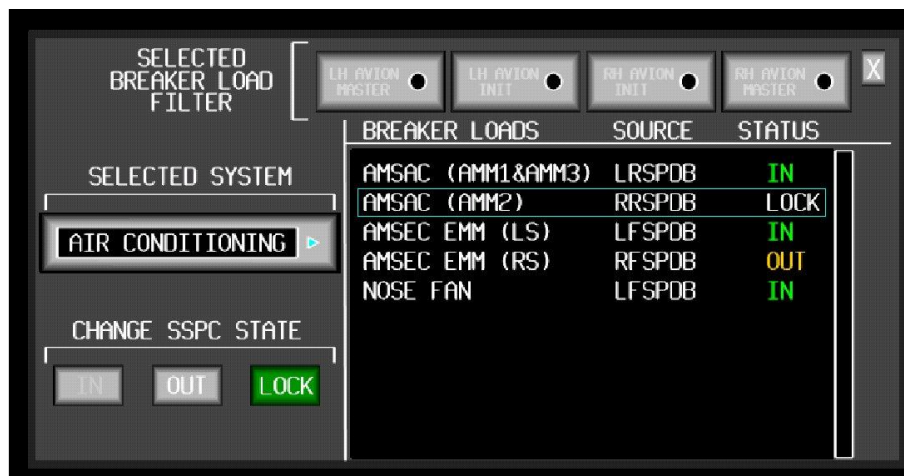
FIGURE 02-24-20-11 – AIR CONDITIONING BREAKERS STATUS PAGE ON GROUND ONLY
