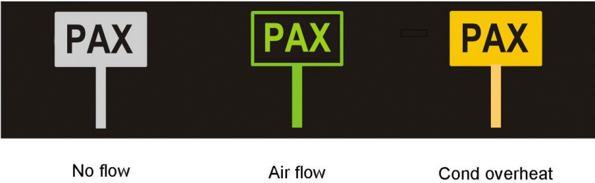
FIGURE 02-36-20-02 - COCKPIT SYMBOL COLOR CODE
