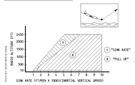
Mode 1 has two boundaries. Penetration of the first boundary generates the illumination of the GPWS lights and a repeated aural alert "SINK RATE". Penetration of the second boundary generates the repetitive "PULL UP".
