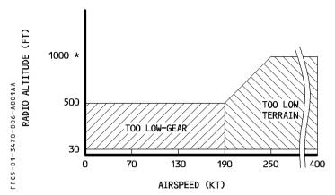
Two aural warnings may be triggered, depending on the area: "TOO LOW-GEAR" or "TOO LOW-TERRAIN". In addition, the GPWS lights come on.
