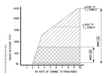
2A — Flaps not in landing configuration and aircraft not on the glide slope beam. Penetration of the boundary lights up the GPWS lights and sounds the repeated aural alert: "TERRAIN".
