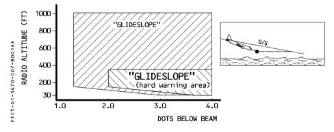
Note: Normally, the GLIDESLOPE alert is only triggered with the gear down. For a few airports, the gear down logic requirement is deleted, and other upper limits are used to increase the warning envelope.
