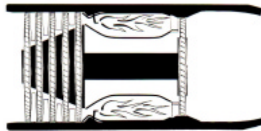
Fig 5 showing basic layout of jet propulsion system.
