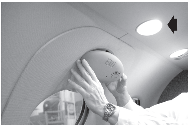
Figure 3-7. Emergency Exit Light
