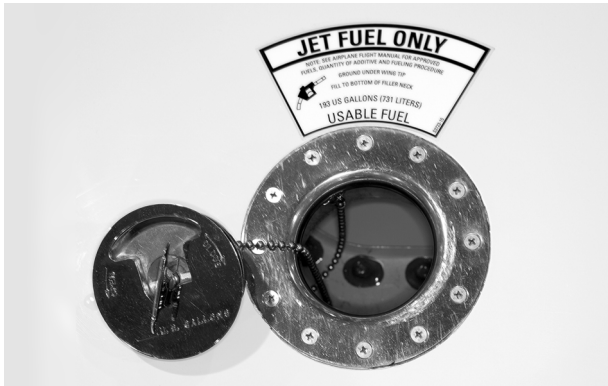
Figure 5-3. Fuel Tank Filler
