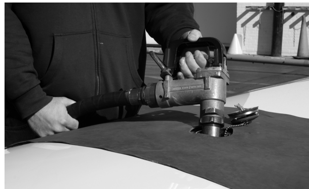
Figure 5-5. Fuel Tank Servicing
