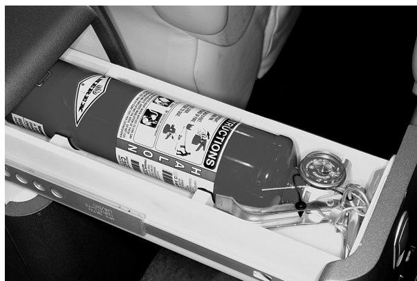
Figure 8-3. Portable Fire Extinguisher
