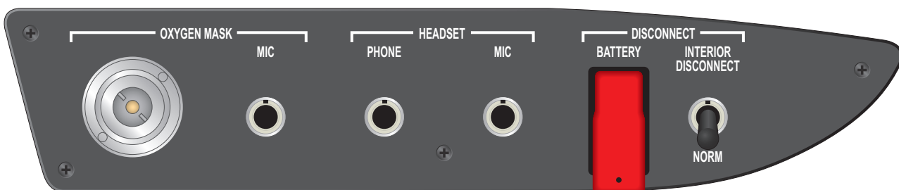
Figure 2-3. Battery Disconnect Switch
