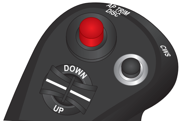
Figure 16-40. Control Yoke Switches
