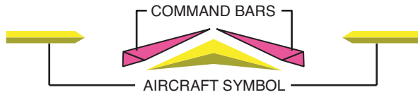
Figure 16-13. Flight Director Single-Cue Command Bars
