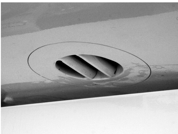
Figure 11-8. Fresh Air Inlet
