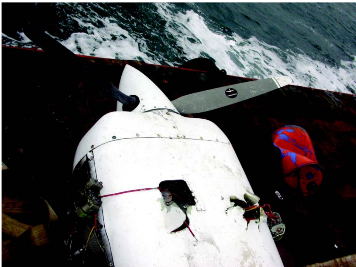
Figure 3. Exterior of the upper outboard engine cowling.
