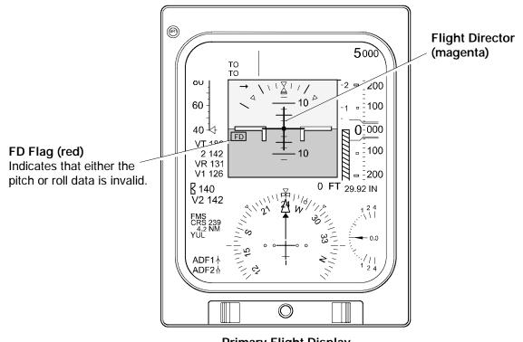
Primary Flight Display Pilot's and Copilot's Instrument Panels
