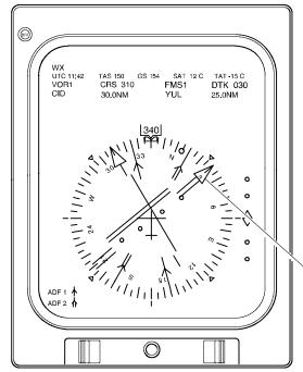
Multifunction Display - HSI Mode Pilot's and Copilot's Instrument Panels
