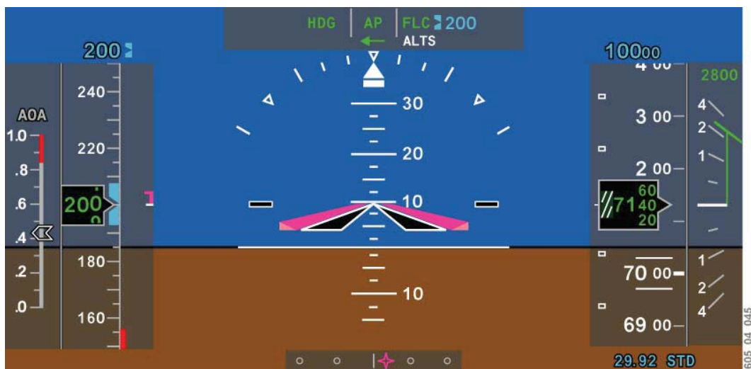
Flight Level Change Mode Figure 04-10-33
