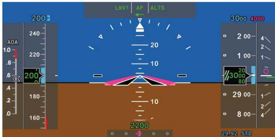
Altitude Capture Sequence Figure 04-10-29
