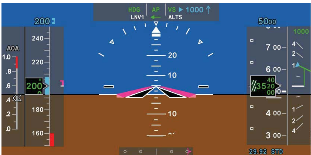
Vertical Speed Mode Figure 04-10-32
