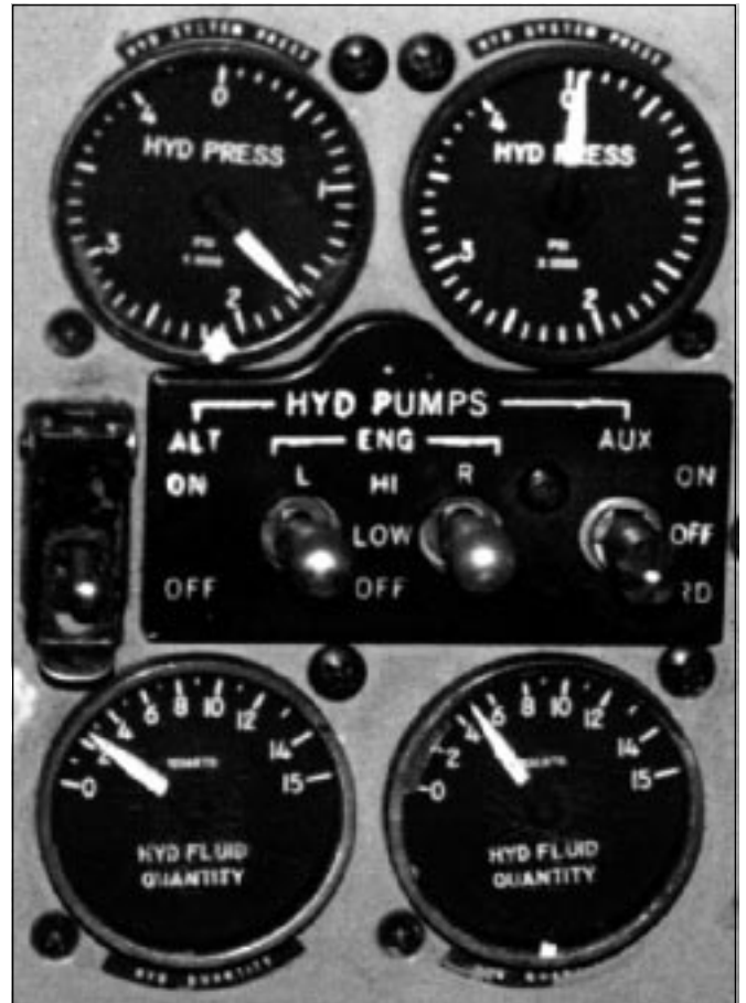
Accident airplane's hydraulics panel in low-pressure configuration. (Photo: U.S. National Transportation Safety Board)
