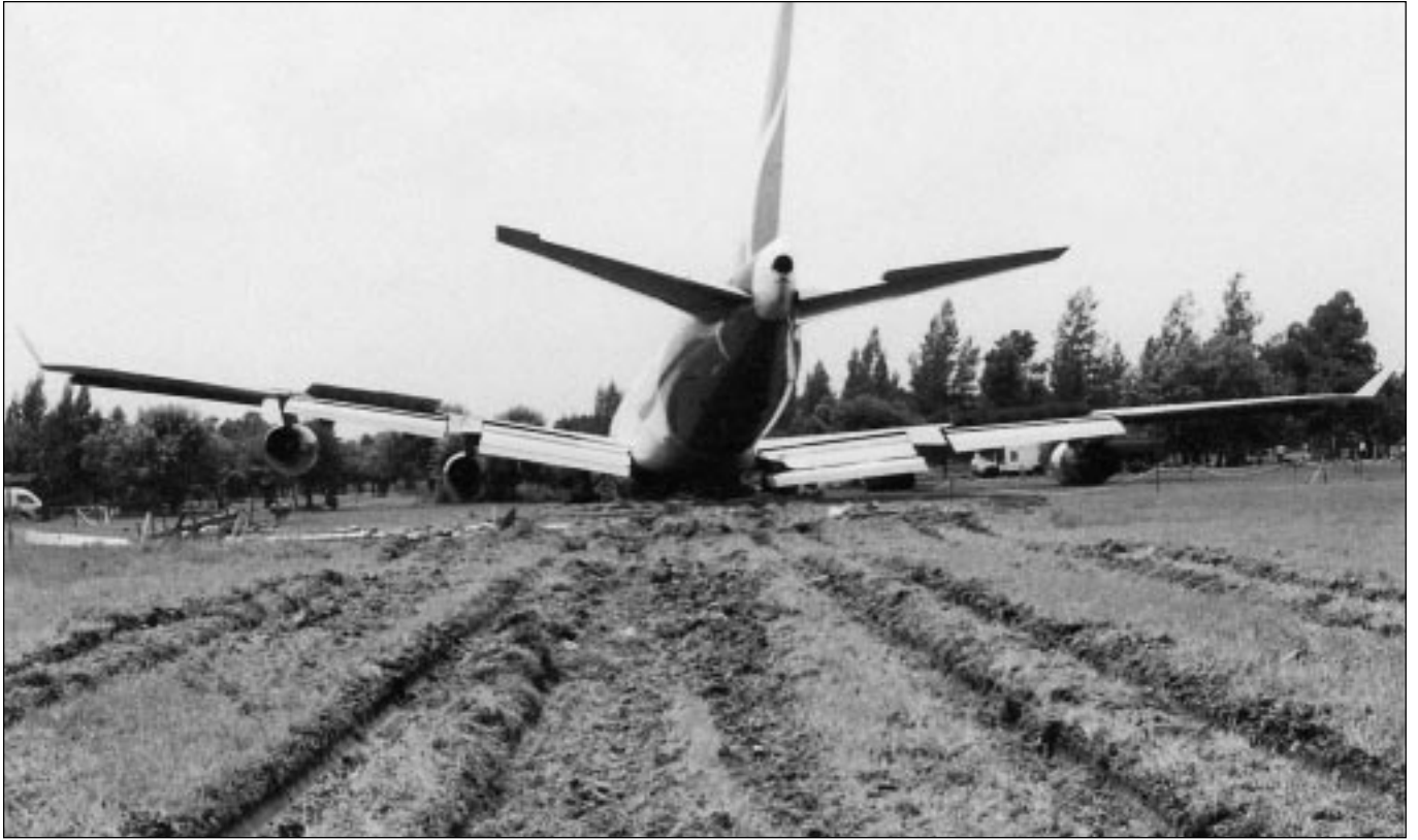
The nose-landing gear and the right-wing landing gear collapsed when the airplane struck the instrument landing system localizer antenna. The airplane continued over wet ground and came to a stop 220 meters (722 feet) from the end of the stopway. (Photo: Australian Transport Safety Bureau)
