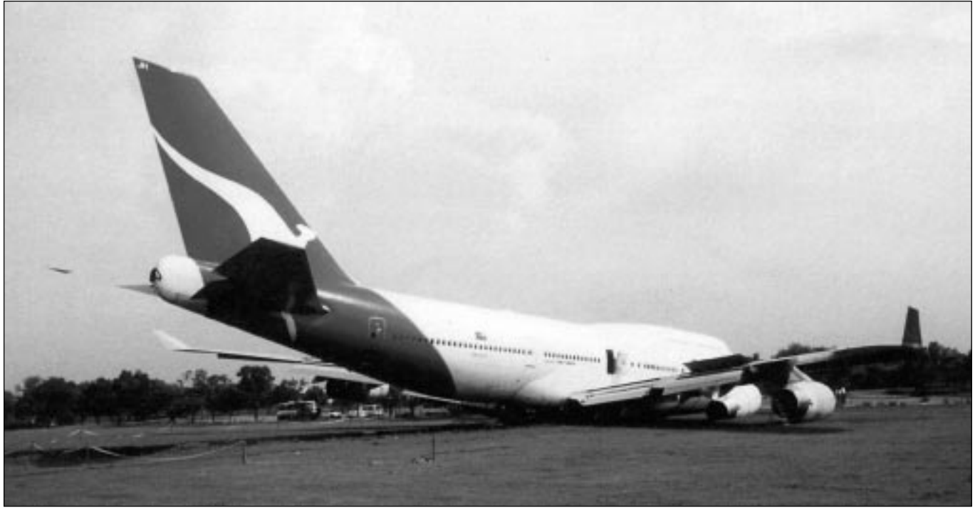
The airplane's landing gear, no. 3 engine nacelle and lower fuselage were damaged during the runway overrun. The airplane came to rest with its nose on an airport-perimeter road. (Photo: Australian Transport Safety Bureau)
