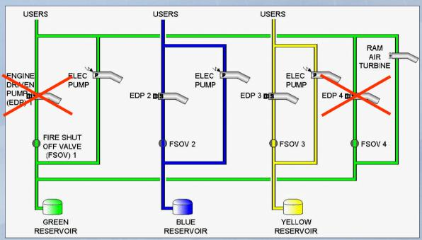
If unserviceable engine is an outer one, additional failure of the other outer prevents gear retraction
