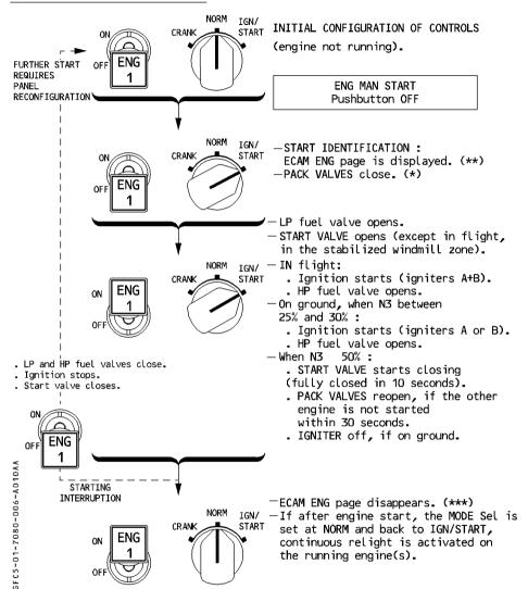
$\underline{\underline{Note}}$ : (\*) If after 30 seconds the engine MASTER switch is not ON, the pack valves will reopen.
