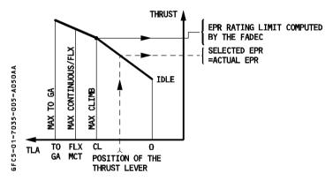
When the thrust lever is set in FLX-MCT detent :
