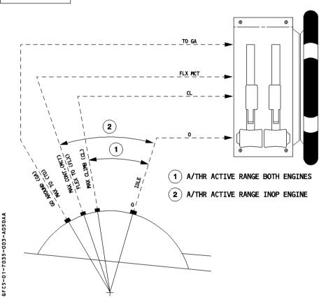
The thrust levers can only be moved manually.
