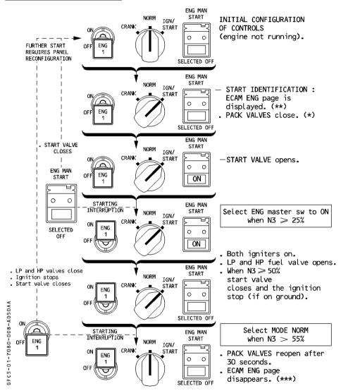
Note: (\*) If after 30 seconds the ENG MAN START pushbutton is not switched ON, the pack valves will reopen.
