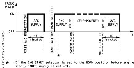
: If the ENG START selector is set to the NORM position before engine start, FADEC supply is cut off.
