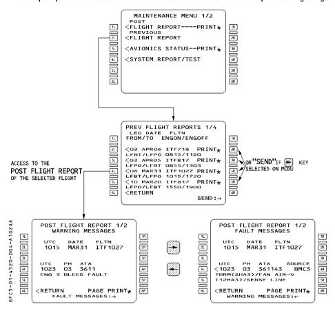
On ground, the operator can either print a flight report or a screen copy. The format is identical to that of the POST FLIGHT REPORT. The operator can send a flight report to the airline ground computer by selecting the corresponding SEND key.
