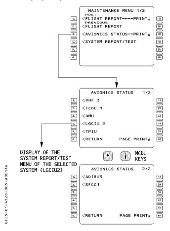
In flight, or on ground, the operator can either print the complete AVIONICS STATUS report, or only a copy of the screen.
