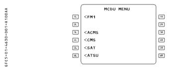
Message/reports are processed by the AOC peripherals (FMS, ACMS, CMS); the ATSU communication function only routes the request according to the company routing policy.
