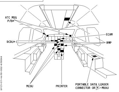
The pilot interface is made of :
