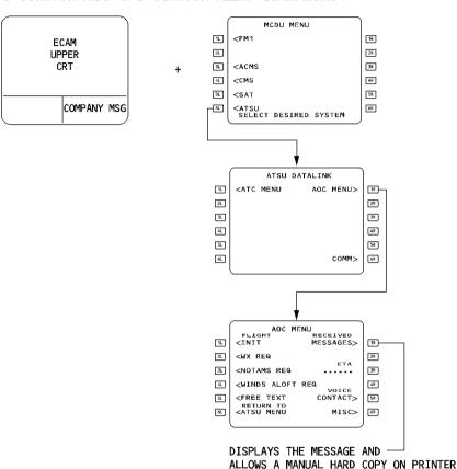
On the AOC MENU page, pressing the [1R] key displays the received message and clears the ECAM memo.
