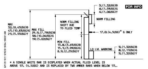
Note: The normal filling range indication is corrected for fluid temperature effect.
