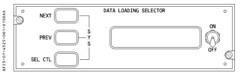
When the data loading selector is ON, the 3 keys (NEXT, PREV, SEL CTRL) enable the display and selection of various applicable aircraft systems (FMGC, TCAS  $\triangleleft$  etc...).
