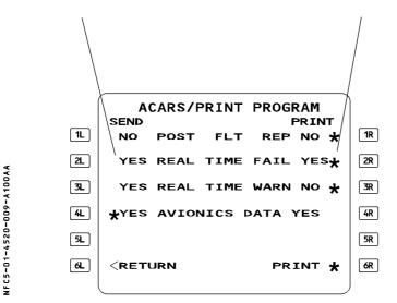
Note: The CFDIU memorizes all manual programming so that at initialisation the last configuration will be retained.
