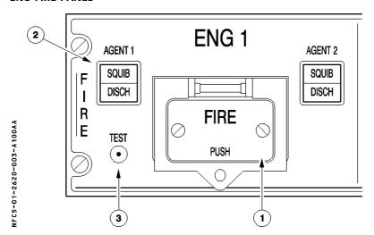
The aircraft has two identical ENG FIRE panels, which contain the following switches and indicators:
