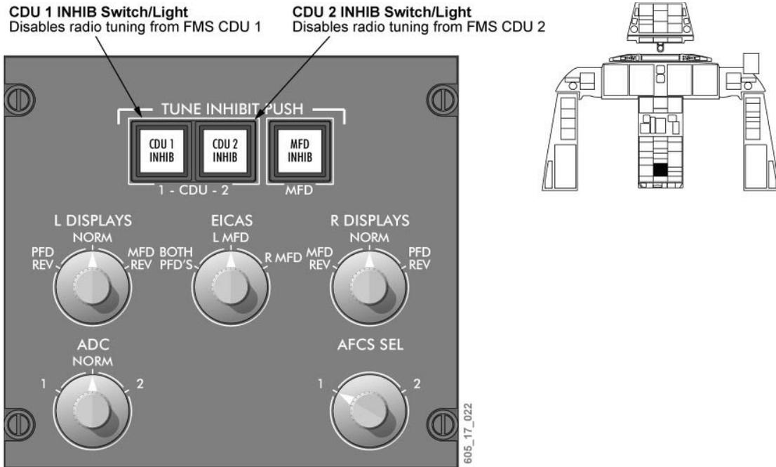
FMS TUNE INHIB Switch/Light
