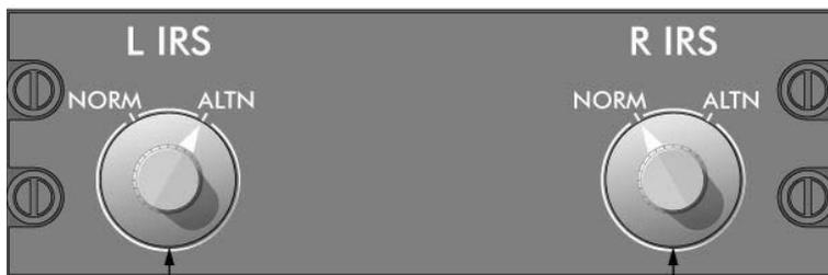
**L IRS Reversionary Mode Selector Switch**
