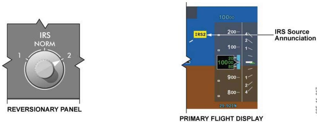
IRS Reversionary Annunciation (Dual IRS Configuration)
