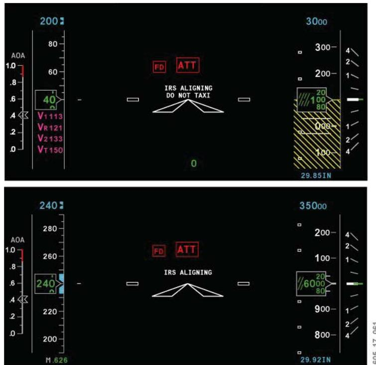
PFD IRS Aligning Annunciations
