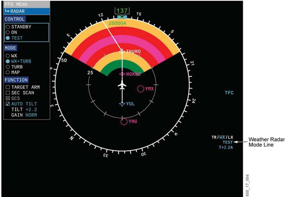
Weather Radar Test Display
