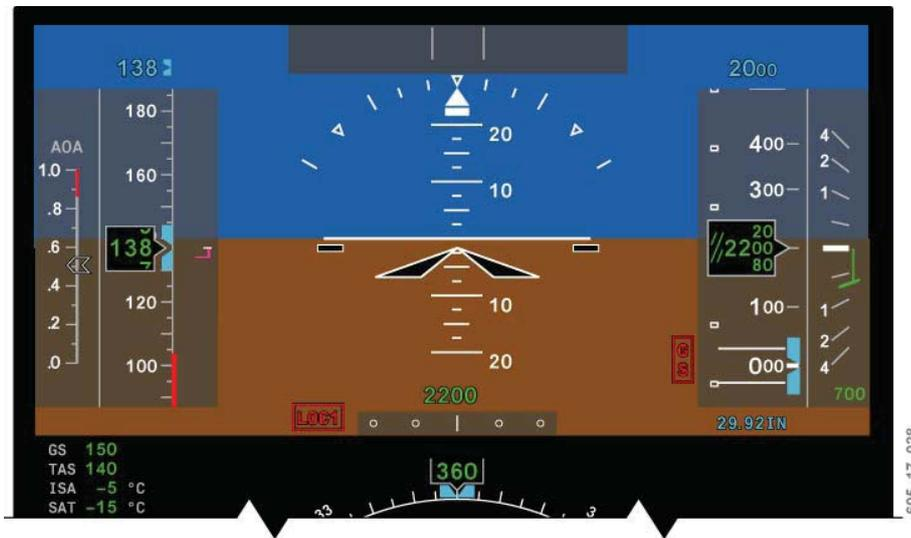
LOC/GS Failure Indications
