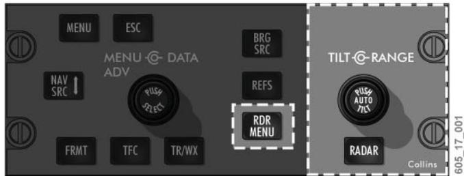
Display Control Panel (DCP) – Weather Radar Controls
