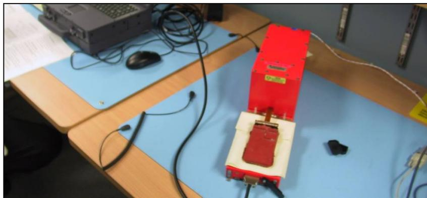
**Figure 6: PK-GZC memory board connected to ATSB SSFDR and RPGSE**
