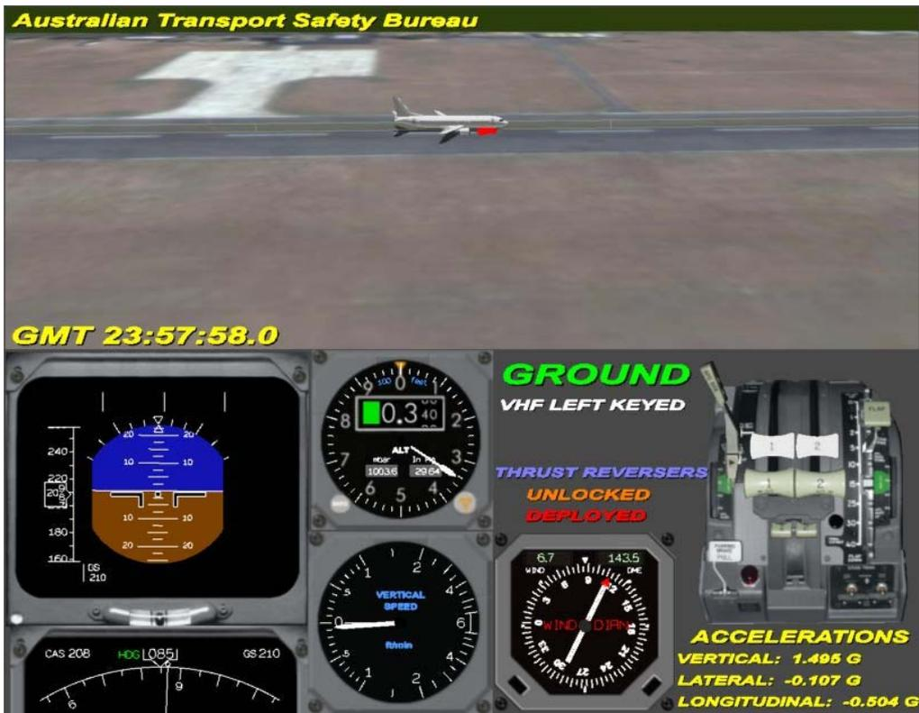
Figure 14: Flight path animation showing start of nose gear scrape
