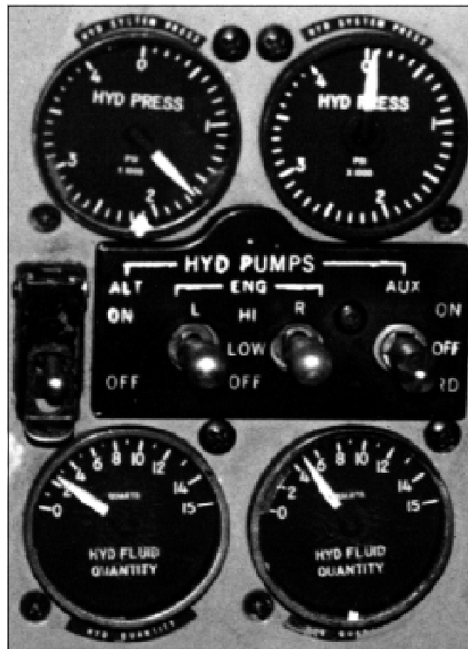
Accident airplane's hydraulics panel in low-pressure configuration. (Photo: U.S. National Transportation Safety Board)
