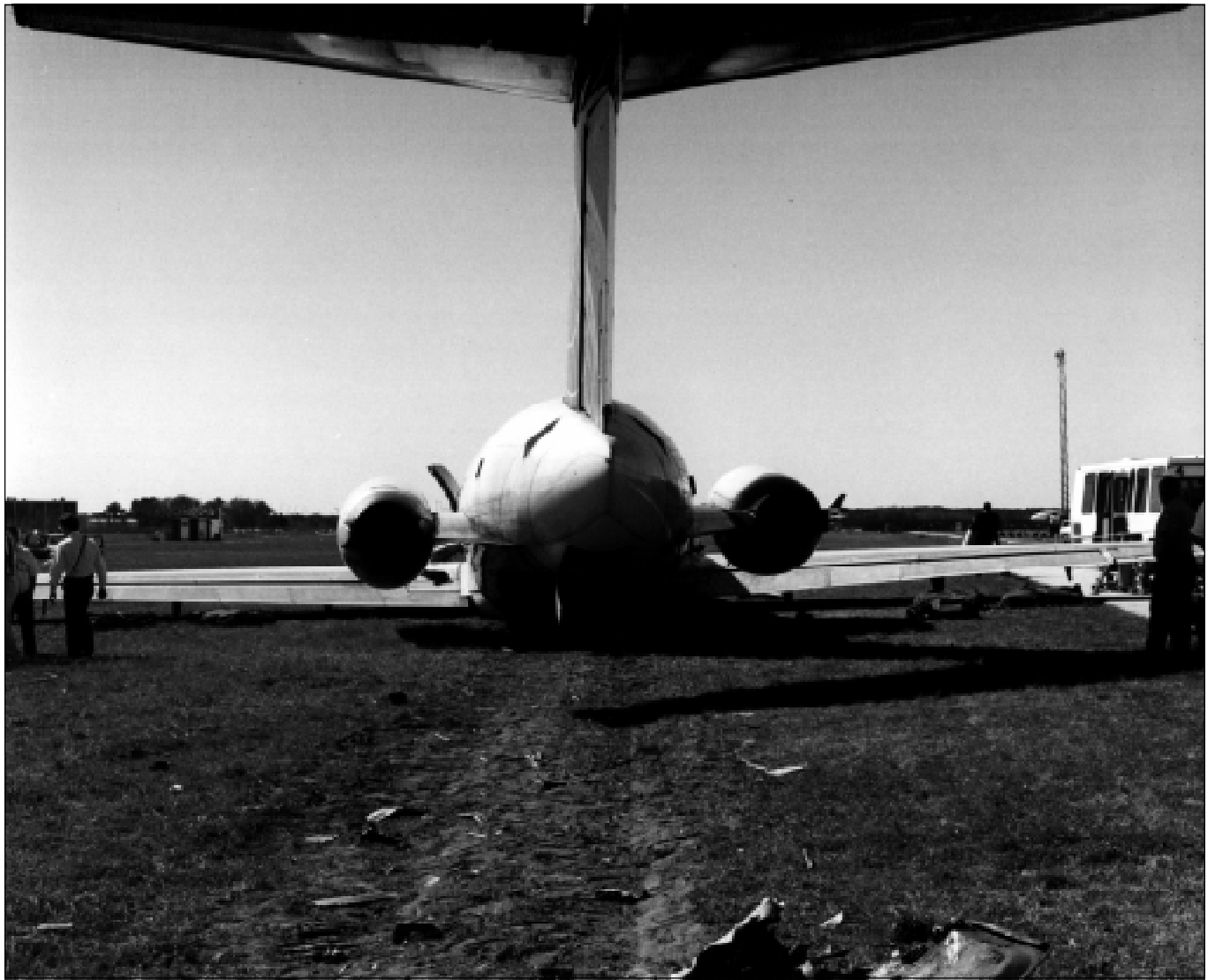
After a wheels-up landing, the Continental Airlines DC-9-32 continued on a trajectory close to the runway centerline for 1,525 meters (5,000 feet), then departed the left side of the runway. The aircraft stopped on the grass adjacent to the upwind end of the runway. (Photo: U.S. National Transportation Safety Board)
