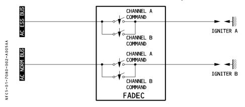
Note: Supply for igniter A switches to the STAT INV BUS BAR as soon as the static inverter is operative.
