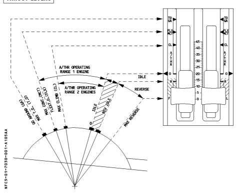
The thrust levers can only be moved manually.
