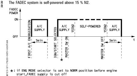
\*: if ENG MODE selector is set to NORM position before engine start, FADEC supply is cut off
