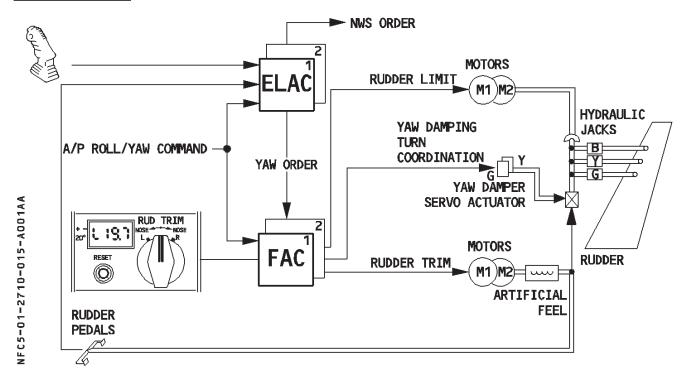
One rudder surface controls yaw.
