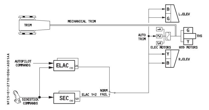
Two elevators and the Trimmable Horizontal Stabilizer (THS) control the aircraft in pitch. The maximum elevator deflection is 30° nose up, and 17° nose down. The maximum THS deflection is 13.5° nose up, and 4° nose down.
