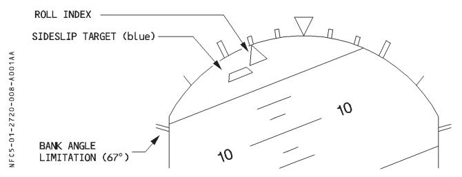
R In flight, the lateral normal law commands some rudder surface deflection to minimize the sideslip. The pilot's response is normal and instinctive: zero the slip indication by applying the right amount of rudder to get the best climb performance.
