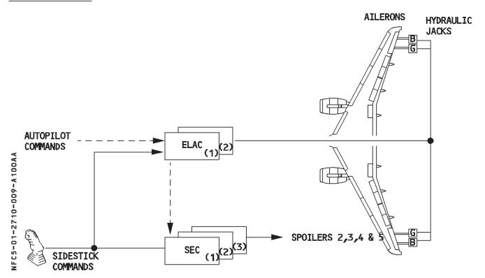
One aileron and four spoilers on each wing control the aircraft about the roll axis. The maximum deflection of the ailerons is 25°.
