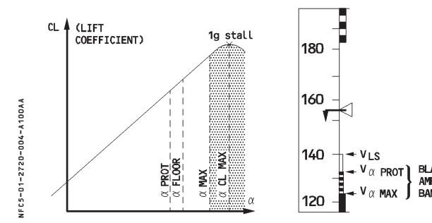
$V\alpha$  prot,  $V\alpha$  floor,  $V\alpha$  max vary according to the weight and the configuration.
