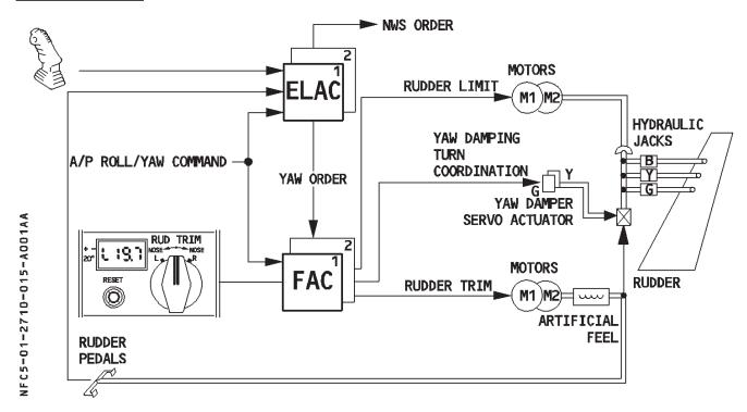
One rudder surface controls yaw.
