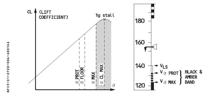
$V\alpha$  prot,  $V\alpha$  floor,  $V\alpha$  max vary according to the weight and the configuration. To deactivate the angle of attack protection, the pilot must push the sidestick :
