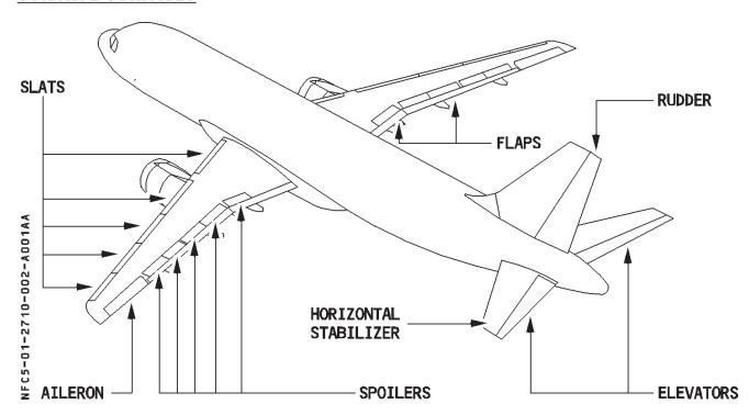
The flight controls are electrically or mechanically controlled as follows:
