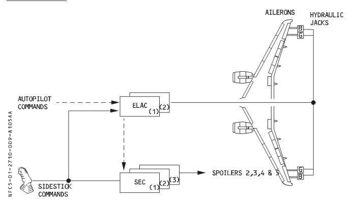
One aileron and four spoilers on each wing control the aircraft about the roll axis.
