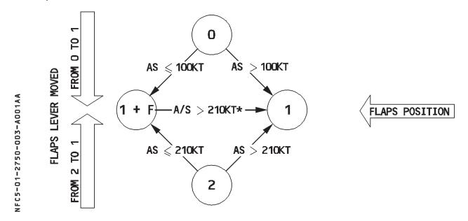
\* When Configuration 1 + F is selected, the flaps retract to 0° automatically at 210 knots (before the airspeed reaches VFE).
